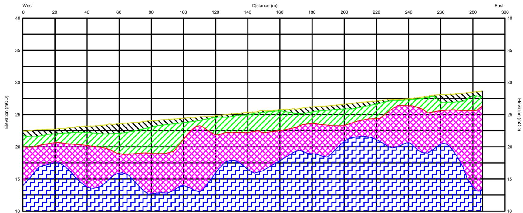
Seismic Refraction Line 2 (S9 - S6) Interpretation
