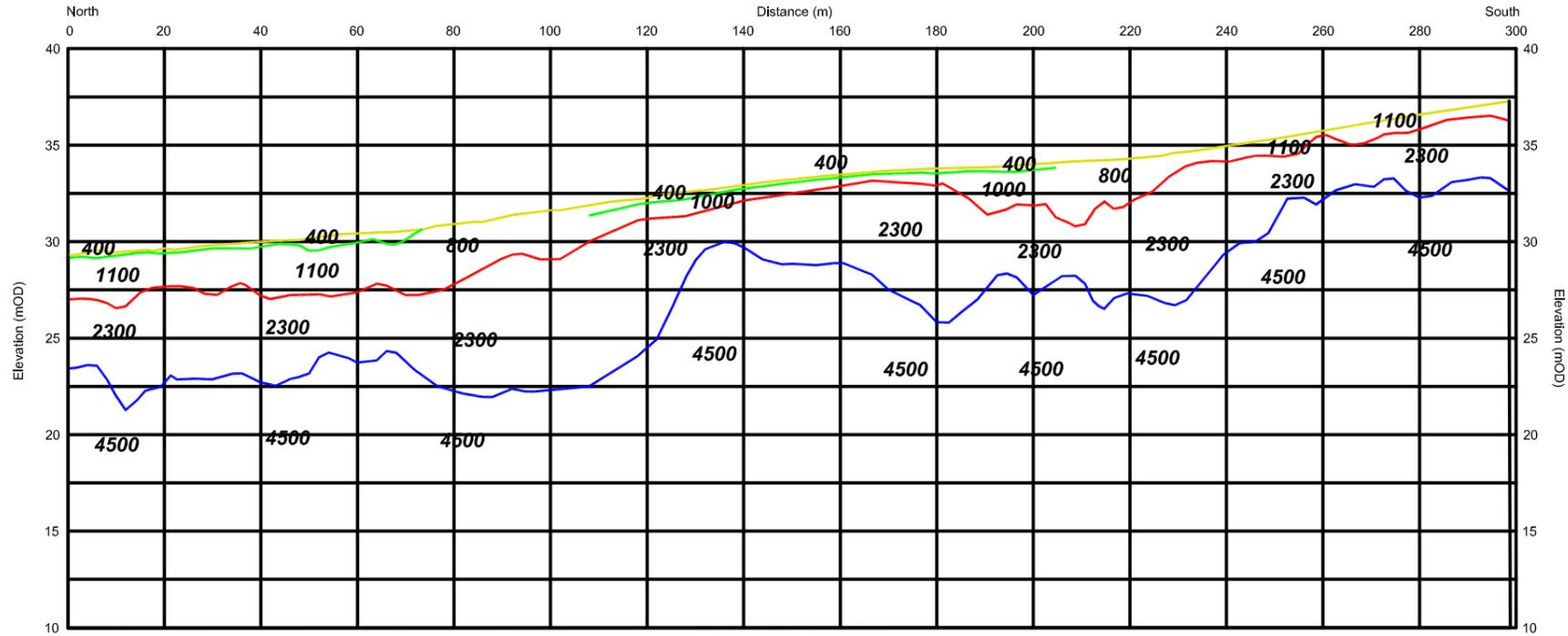
Seismic Refraction Line 6 (S1 - S5) Model
