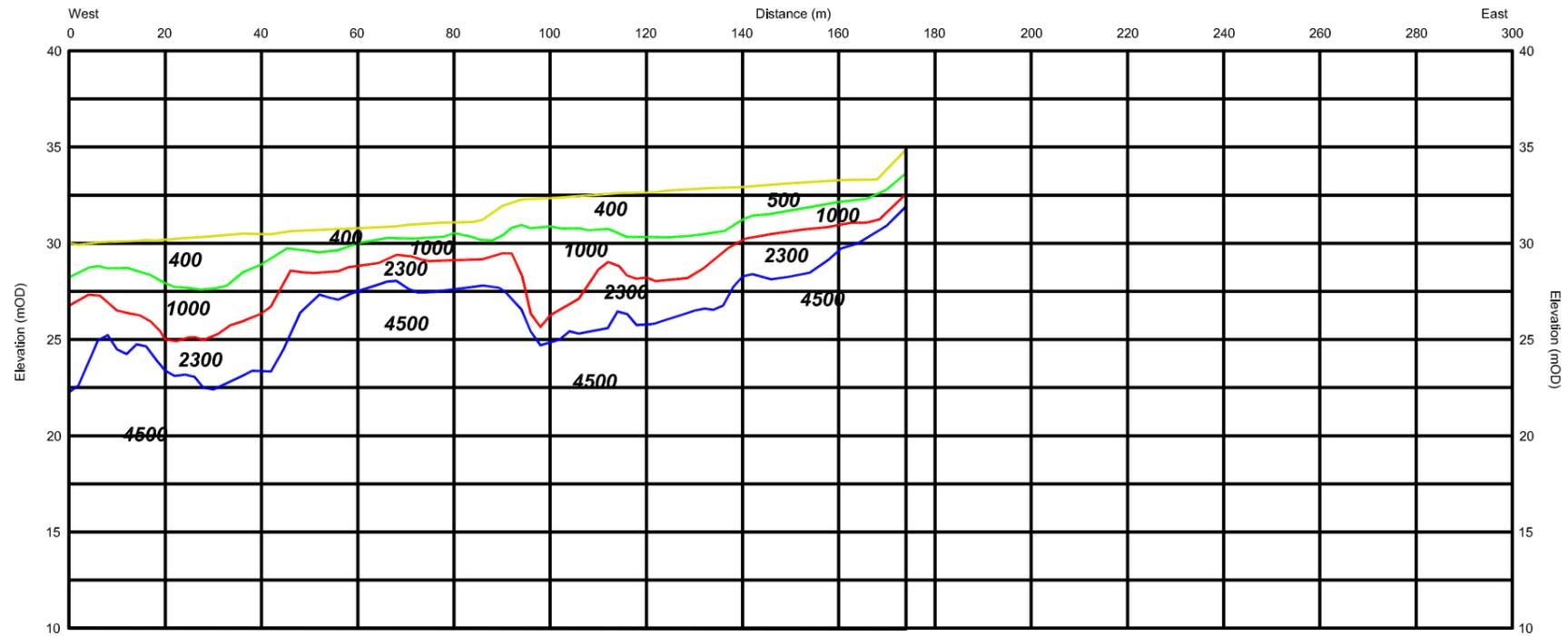
Seismic Refraction Line 3 (S12 - S14, S18 - 19) Model
